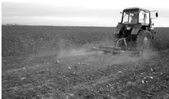
Fig. 1. ISX 3.6 cotton stalk chopper is in the field [6]
