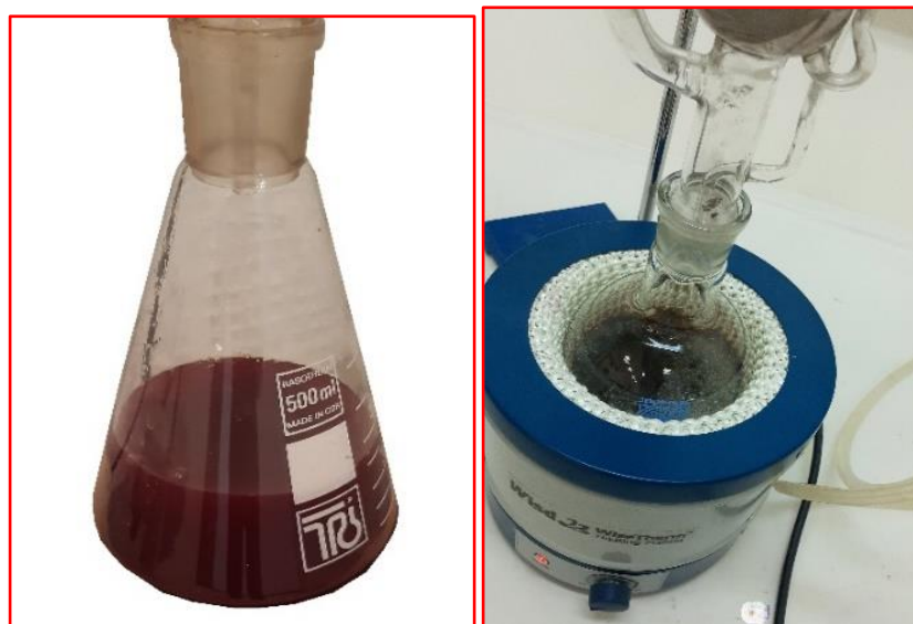
Fig. 1. Soxhlet extraction and blackberry extract
