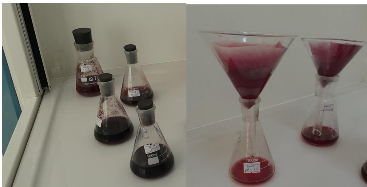
Fig.3. Ready anthocyanin extraction and filtering part of natural pigment
